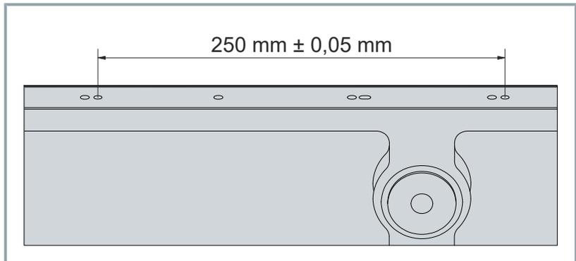
The distance between the center of the first locating pin bore for one module to the center of the first locating pin bore for the next module must be 250 mm. The manufacturing tolerance is  $\pm 0.05$  mm.
