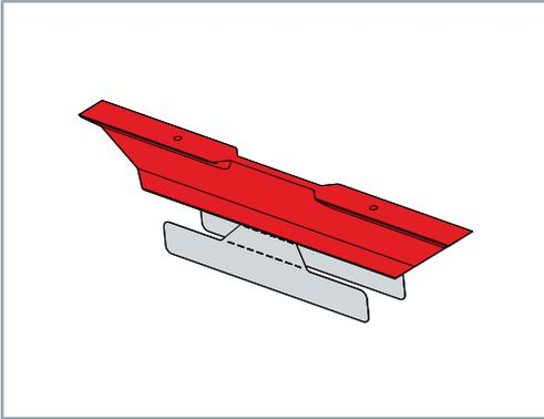
The XTS Hygienic movers are mounted on the guide rail by means of the rail on support.
