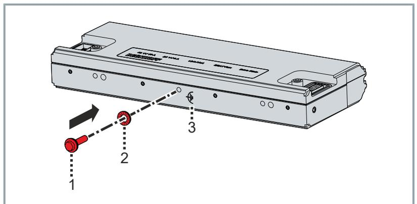
When screwing the screw with seal 1 into the tapped hole with the marking "functional earth" 3, use a contact washer 2 between the machine bed and the seal.
