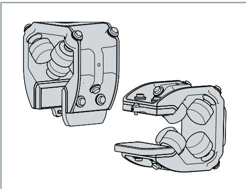
The stainless steel mover is 75 mm long, has 6 rollers and is mounted with a magnetic plate set.
