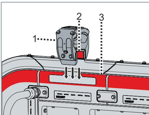
As soon as you place the magnetic plate set 2 of the mover 1 in the vicinity of the module 3, the magnetic plate set and the module attract each other magnetically.
