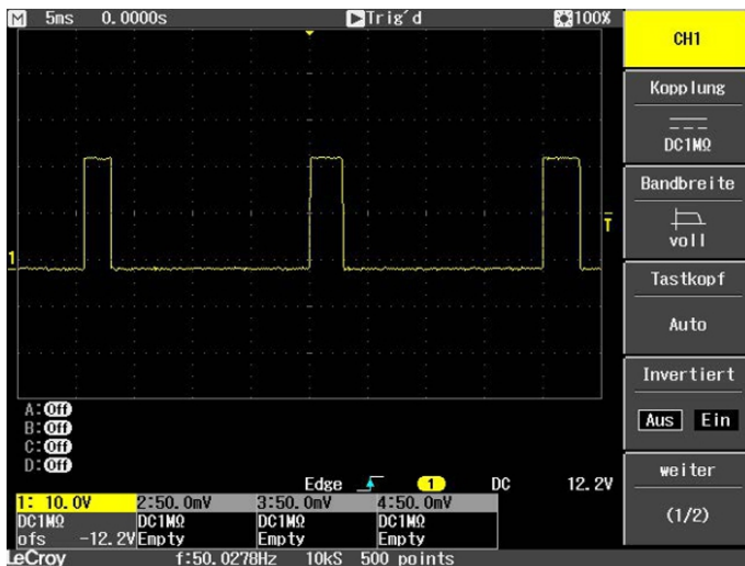
Fig. 41: Shortened pulse of a digital output with load.
