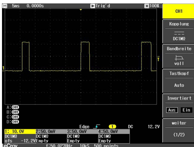
Fig. 38: Shortened pulse of a digital output with load.
