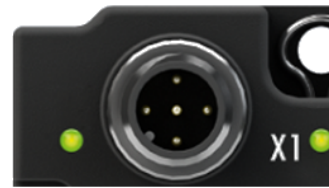
IO-Link Device status LED (wide housing)
