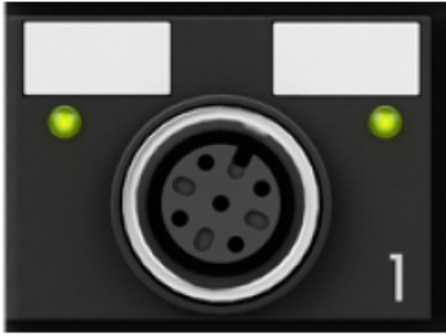
Fig. 8: IO-Link connection, master
