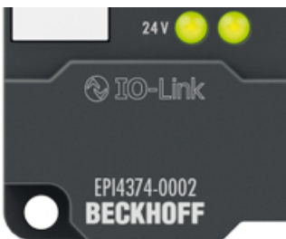
Fig. 10: Status LEDs for power supply
