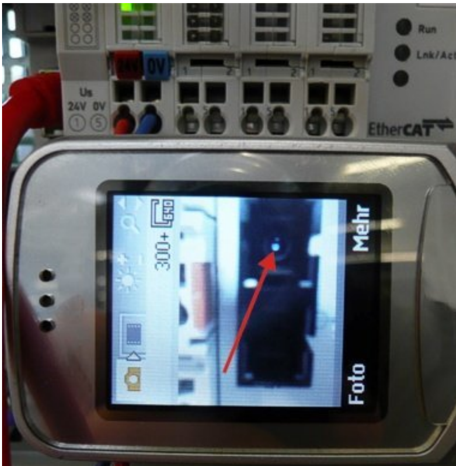
Fig. 27: Visualization of infrared light at the SC duplex connector
