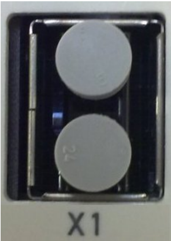
Fig. 31: Blind plugs in unused sockets
