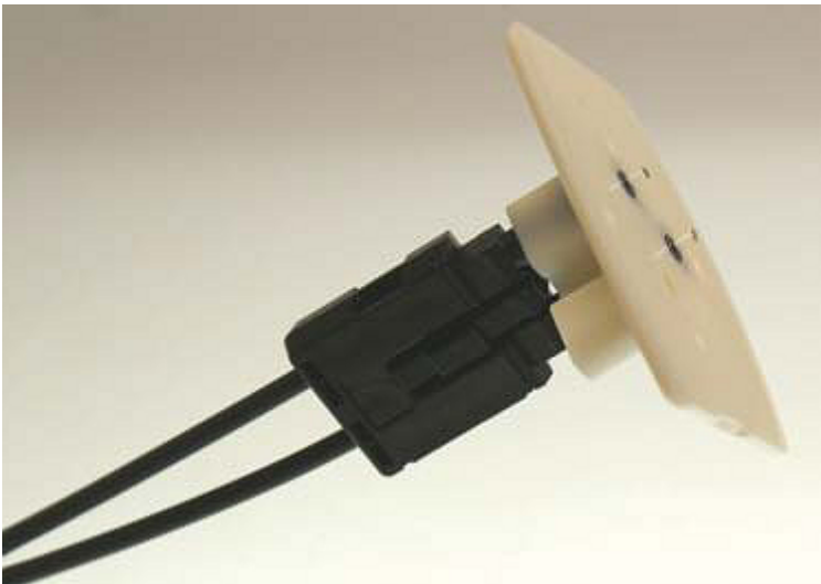
Fig. 37: Sanding gauge with protruding fiber ends
