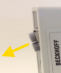
Fig. 23: Slanting installation of the optical fiber socket
