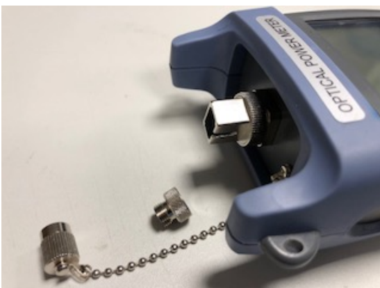
OPM with SC adapter screwed on
