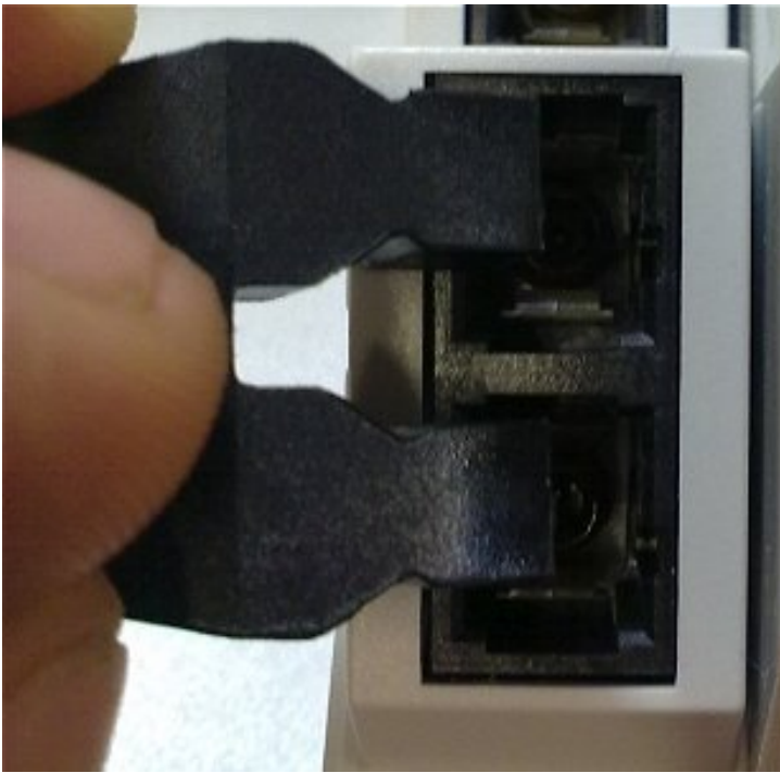
Fig. 28: Blind plugs in unused sockets
