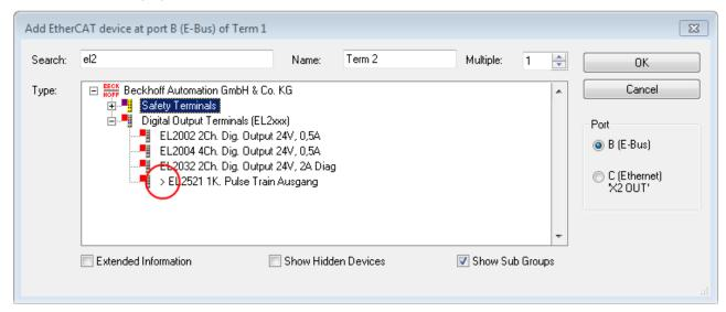
Fig. 72: Indication of an online recorded ESI of EL2521 as an example
