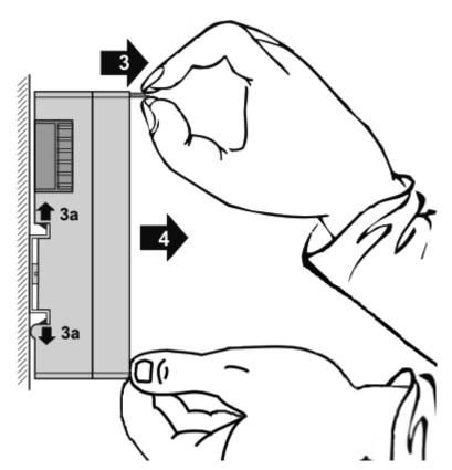
• Pull (4) the terminal module away from the mounting surface.
