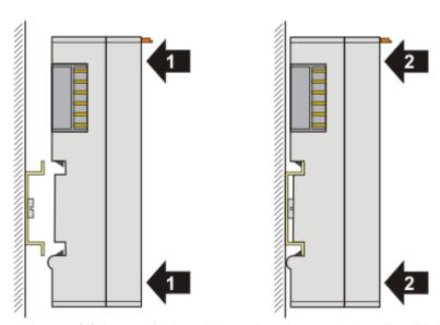
and press (1) the terminal module against the mounting rail until it latches in place on the mounting rail (2).
