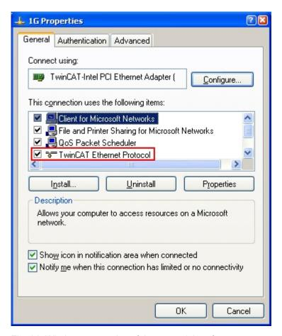
Fig. 64: Windows properties of the network interface
