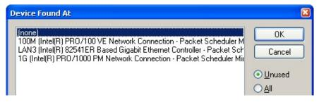
Fig. 76: Selecting the Ethernet port
