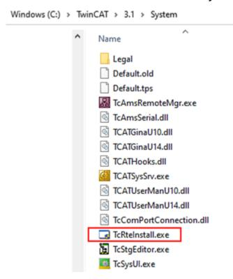
Fig. 61: TcRteInstall in the TwinCAT directory
