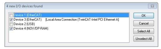
Fig. 87: Detected Ethernet devices
