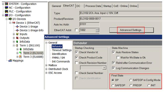
Fig. 120: Default target state in the Slave
