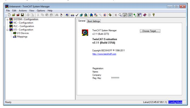
Fig. 19: Initial TwinCAT 2 user interface
