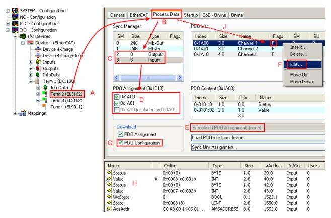
Fig. 109: Configuring the process data
