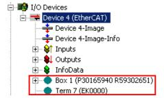
Fig. 98: Faulty identification
