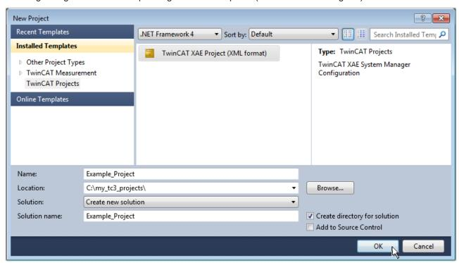
Fig. 37: Create new TwinCAT project
