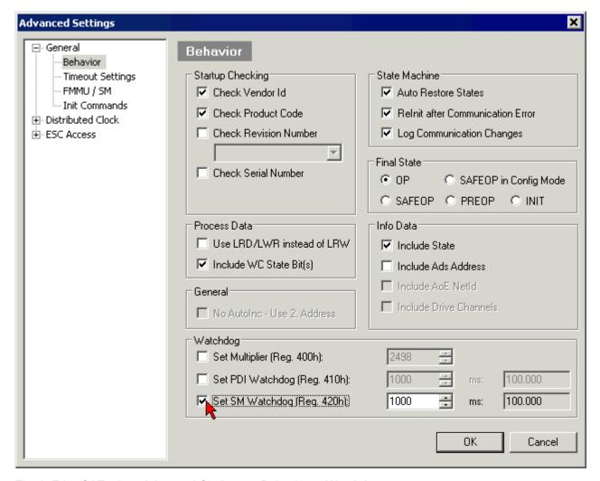
Fig. 6: EtherCAT tab -> Advanced Settings -> Behavior -> Watchdog
