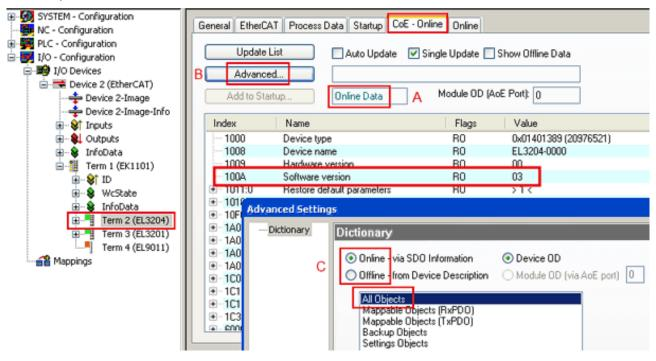
Fig. 139: Display of EL3204 firmware version
