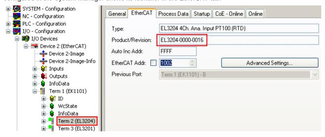
Fig. 133: Device identifier consisting of name EL3204-0000 and revision -0016
