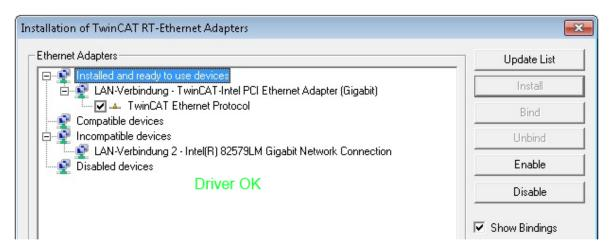
Fig. 65: Exemplary correct driver setting for the Ethernet port
