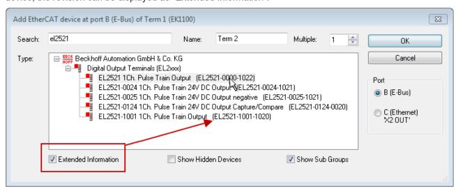
Fig. 80: Display of device revision
