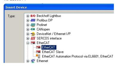
Fig. 59: Selecting the EtherCAT connection (TwinCAT 2.11, TwinCAT 3)
