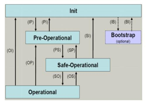
Fig. 30: States of the EtherCAT State Machine
