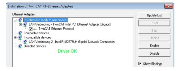
Fig. 49: Exemplary correct driver setting for the Ethernet port
