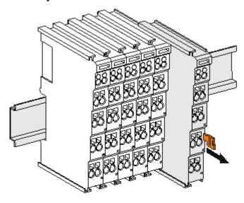
Fig. 33: Disassembling of terminal
