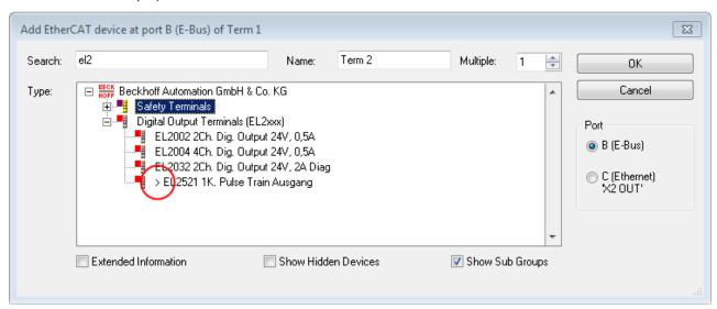
Fig. 56: Indication of an online recorded ESI of EL2521 as an example
