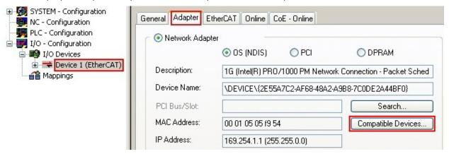
Fig. 47: EtherCAT device properties (TwinCAT 2): click on "Compatible Devices..." of tab "Adapter"
