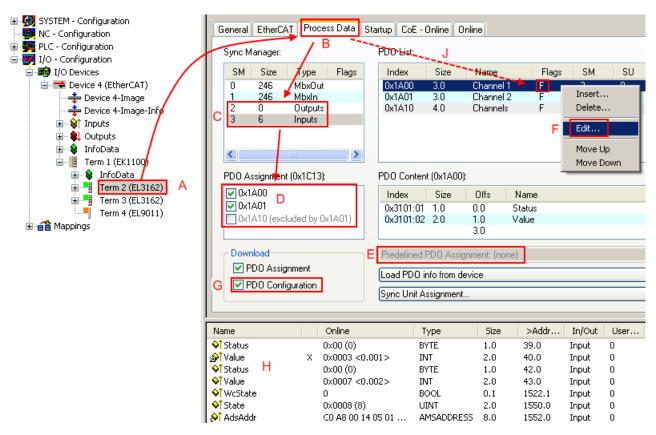
Fig. 89: Configuring the process data
