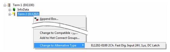
Fig. 88: TwinCAT 2 Dialog Change to Alternative Type
