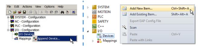
Fig. 58: Append EtherCAT device (left: TwinCAT 2; right: TwinCAT 3)
