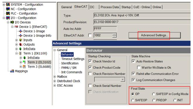
Fig. 99: Default target state in the Slave
