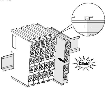
Fig. 32: Attaching on mounting rail
