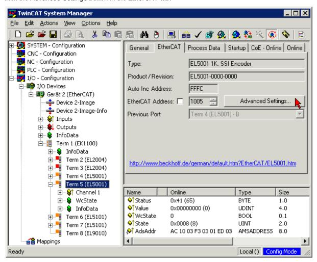
The Advanced Settings dialog appears. Under ESC Access/E<sup>2</sup>PROM/FPGA click on Write FPGA button:
