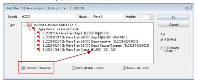
Fig. 64: Display of device revision
