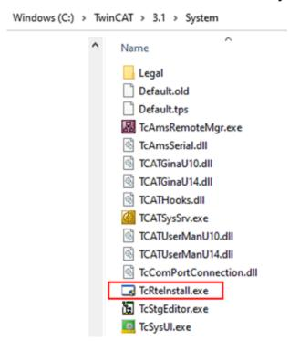
Fig. 45: TcRteInstall in the TwinCAT directory
