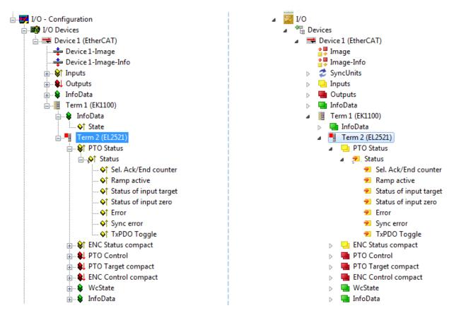
Fig. 67: EtherCAT terminal in the TwinCAT tree (left: TwinCAT 2; right: TwinCAT 3)
