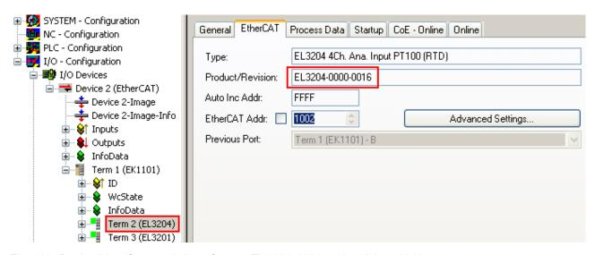
Fig. 103: Device identifier consisting of name EL3204-0000 and revision -0016
