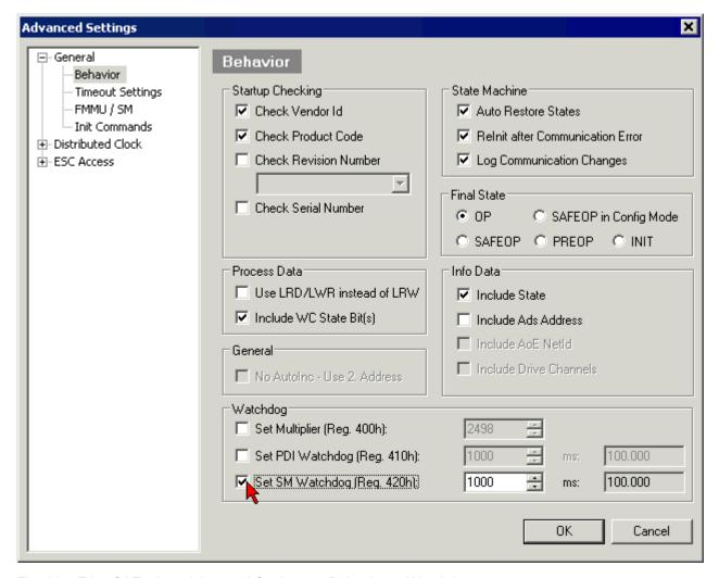
Fig. 29: eEtherCAT tab -> Advanced Settings -> Behavior -> Watchdog
