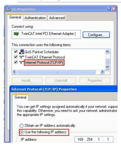
Fig. 51: TCP/IP setting for the Ethernet port
