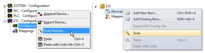
Fig. 69: Scan Devices (left: TwinCAT 2; right: TwinCAT 3)
