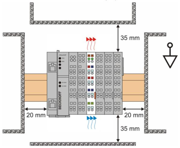
Fig. 37: Recommended distances for standard installation position
