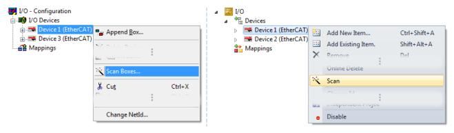
Fig. 76: Manual scanning for devices on a specified EtherCAT device (left: TwinCAT 2; right: TwinCAT 3)
