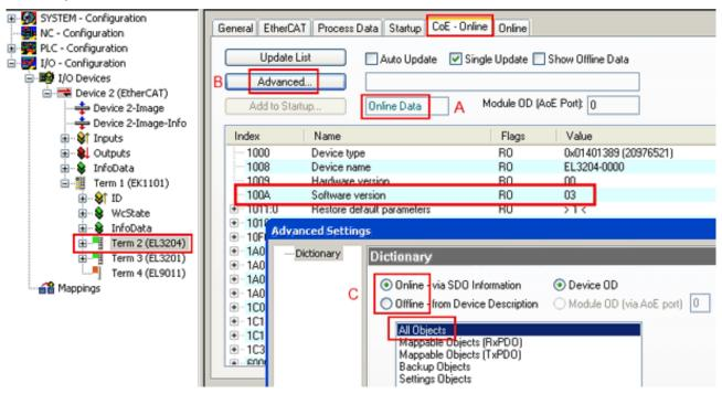
Fig. 109: Display of EL3204 firmware version
