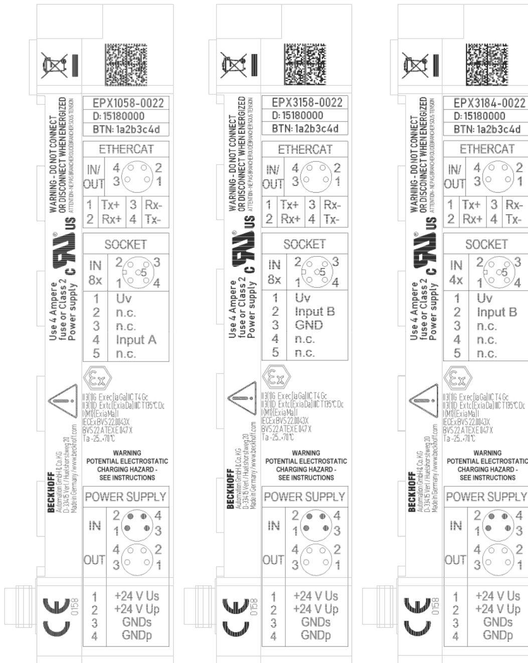
Fig. 1: Side name plate of EPX1058-0022, EPX3158-0022 and EPX3184-0022
