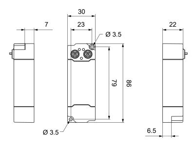
All dimensions are given in millimeters. The drawing is not true to scale.
