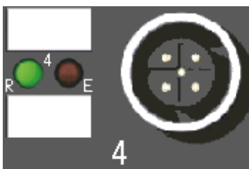
Fig. 4: Status and diagnostic LED at the M12 connector
