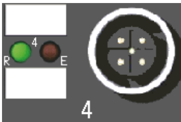
Fig. 5: Status and diagnostic LED at the M12 connector
