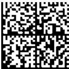
Fig. 22: Example DMC 1P 072222 S BTNk4p562d7 1K EL1809 Q 1 51S 678294
