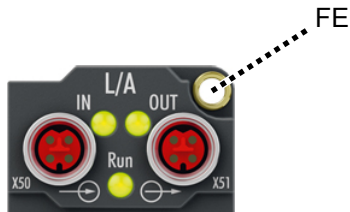
Fig. 1: Connection for functional earth (FE)
