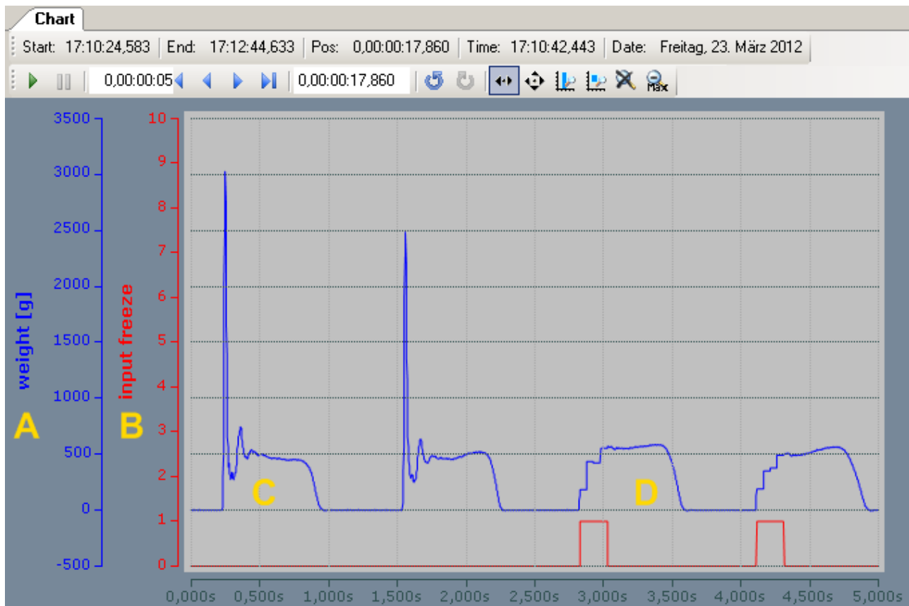
Fig. 13: Impulses on a load cell with and without InputFreeze
