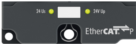
Fig. 10: status-LEDs for the power supply
