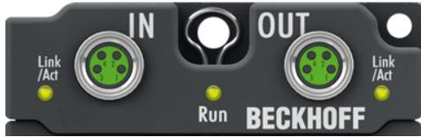
Abb. 6: EtherCAT Status-LEDs
