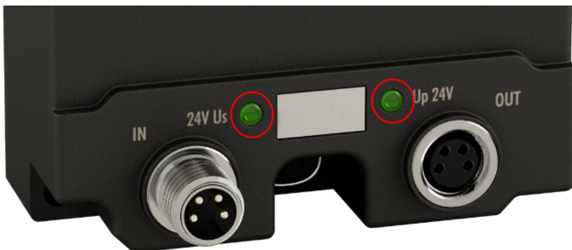
Fig. 15: LED display for the supply voltages
