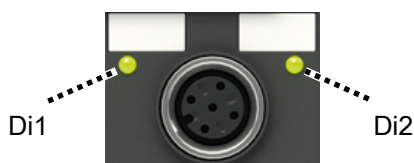
Fig. 18: Status LEDs for limit switch
