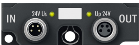
Fig. 9: Status LEDs for the supply voltages
