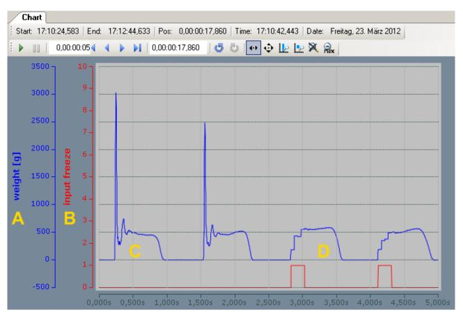
Fig. 18: Impulses on a load cell with and without InputFreeze
