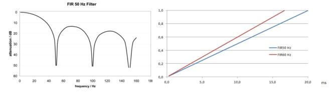
Fig. 4: Notch characteristic/amplitude curve and step response of the FIR filter
