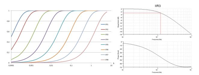
Fig. 5: Step response and Bode diagramm of the IIR filter
