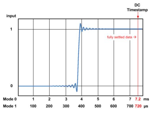
Fig. 7: Latency of the Analog-to-Digital converter
