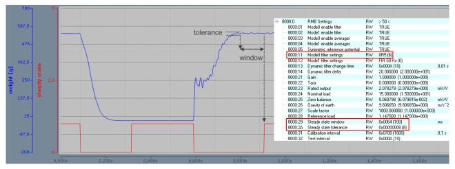
Fig. 19: Abrupt unloading and subsequent reloading of a load cell
