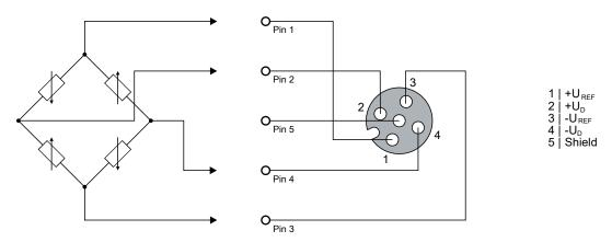
Connect the cable shield to pin 5 of the M12 connector.
