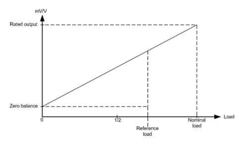
Fig. 20: Adaptation to the sensor curve
