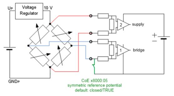
Fig. 17: Internal switch for increasing the measuring accuracy
