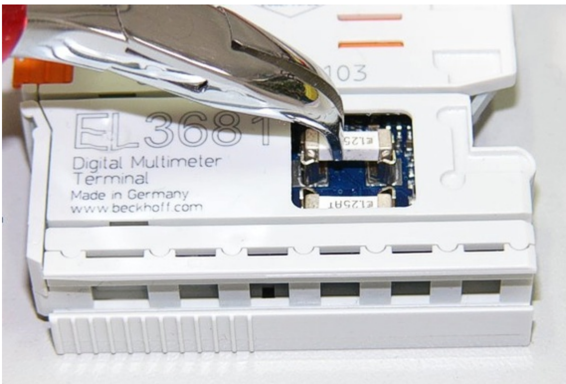
Fig. 32: Replacing the fuse
