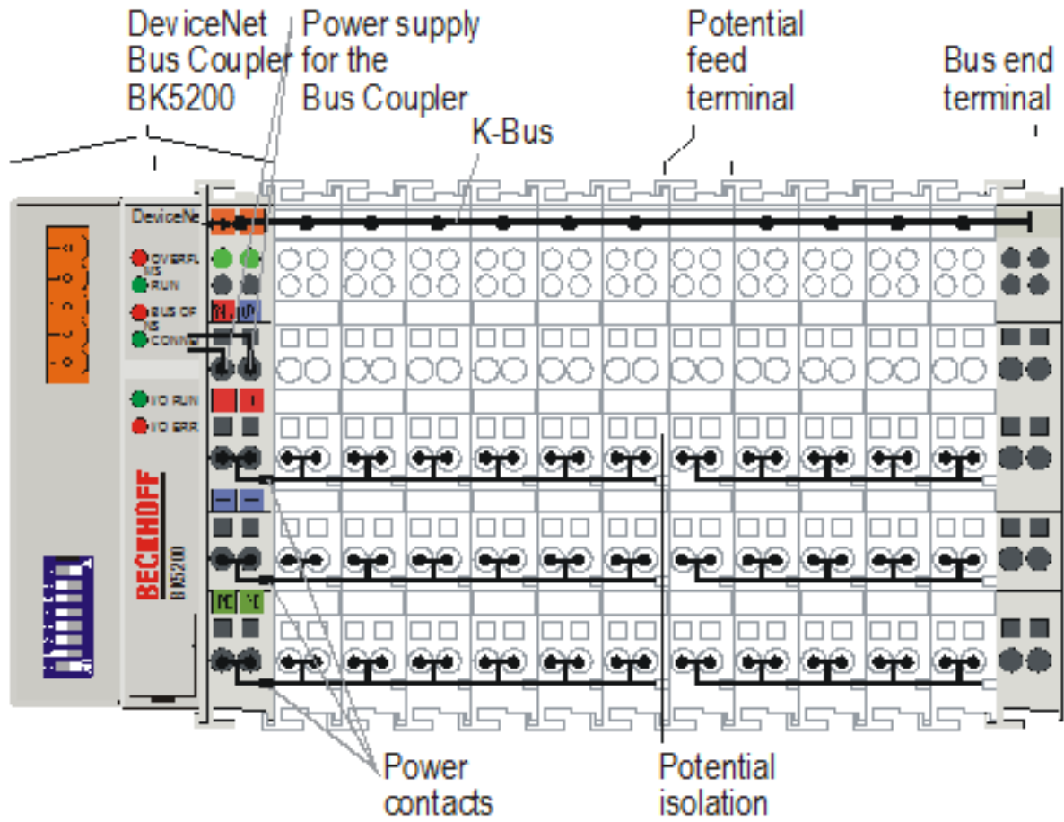
Fig. 4: Principle of the Bus Terminal
