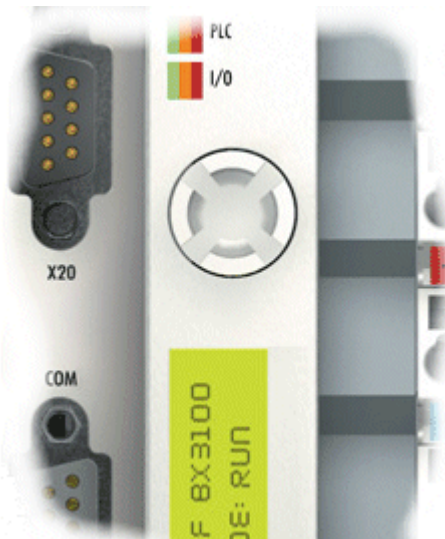
Fig. 84: Navigation switches of the BX controller
