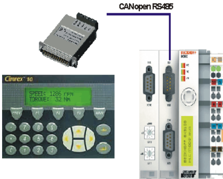
Fig. 72: Cimrex panel at the SSB of the BX controller
