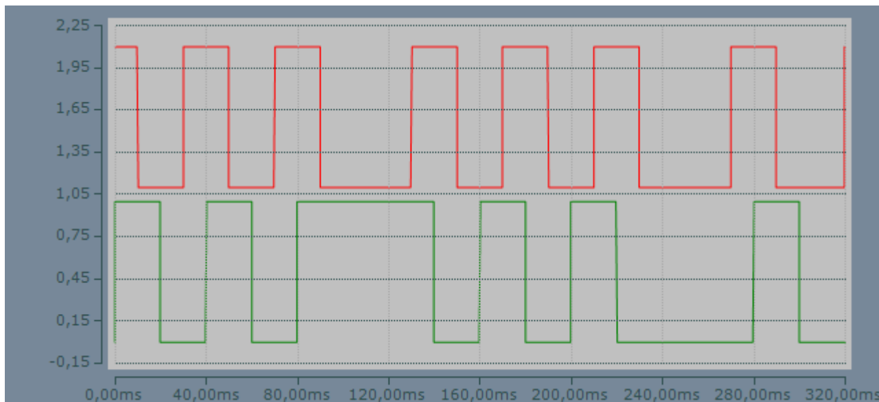
Fig. 27: Example of the signal curve of the input signal in the operating mode Two Channel Encoder Velocity Control
