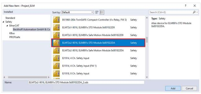
The "Add New Item" window opens and you can select the desired Alias Device. In the name you will find the information about which ELM8911 variant with the associated Moduleldent it is.
