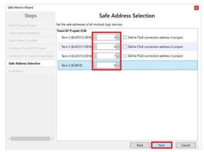
15. In the "Safe Address Selection" window, configure safe addresses of all devices
