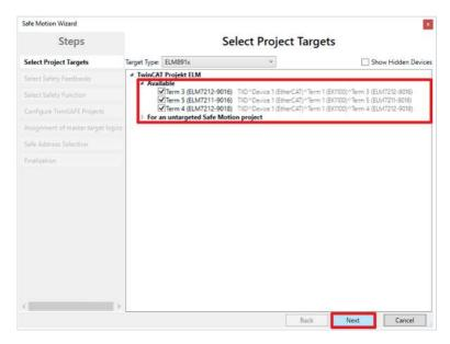
The "Select Project Targets" window shows the existing components and the virtual axes for single-axis and double-axis modules.
