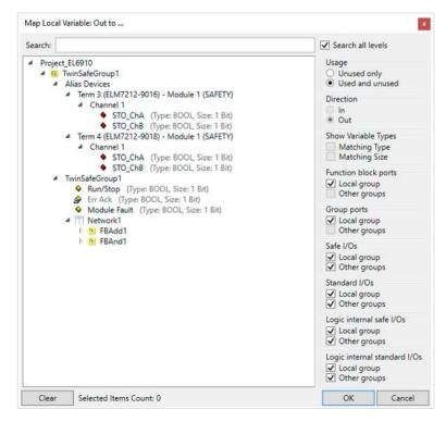
The variables are displayed with the corresponding designation in Variable Mapping.
