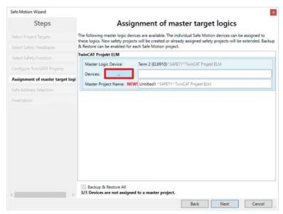
11. Set the master project in the "Assignment of master target logics" window
