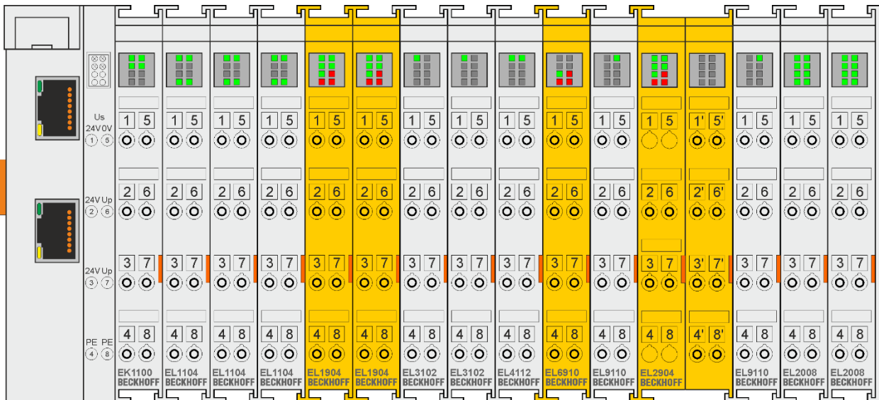
Fig. 4: Sample configuration for temperature measurement
