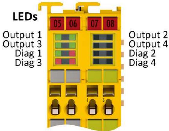
Abb. 24: Diagnose-LEDs
