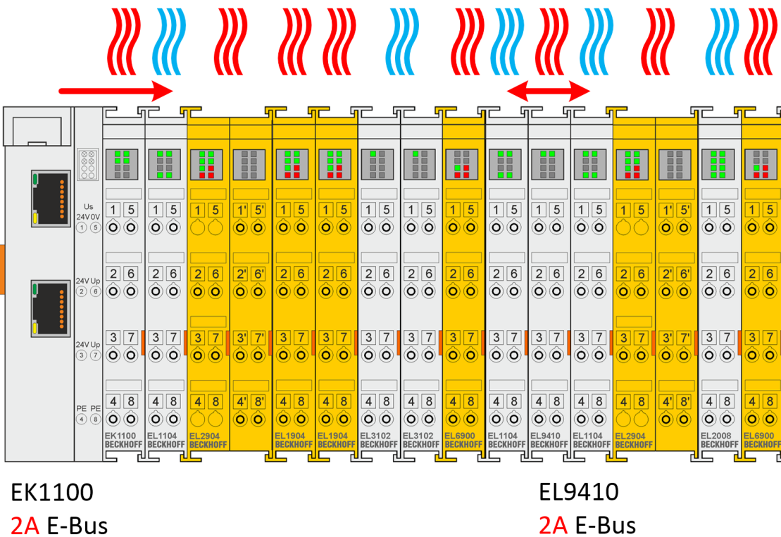
Fig. 10: Thermally favorable arrangement of the TwinSAFE terminals
