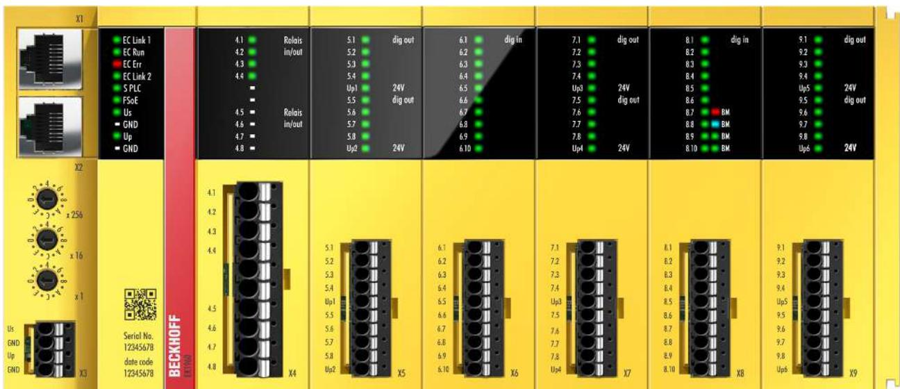
Abb. 1: EK1960-260x TwinSAFE-Compact-Controller
