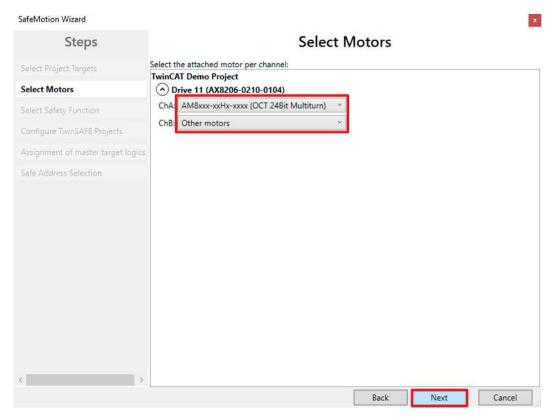
In the "Select Motors" window, configure the feedback for the individual axes.
