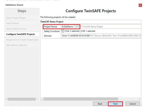
The "Configure TwinSAFE Projects" window opens. Here you have the option of renaming your Safe Motion project, which is generated for your Safe Motion component.
