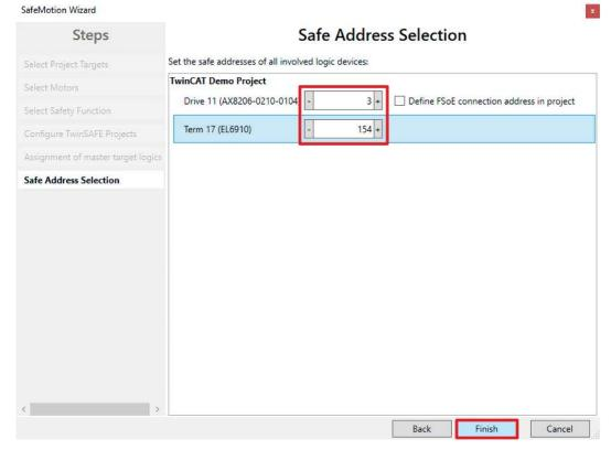
The "Safe Address Selection" window opens. Here the safe addresses are read out automatically. For virtual axes or axes that cannot be reached, you have the option of configuring the addresses yourself.
