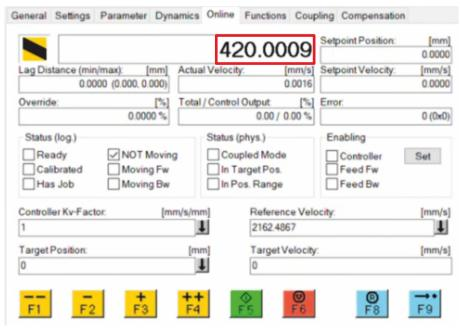
You can see from the configuration that the position is approximately 420 mm. This value is to be configured as the zero point.
