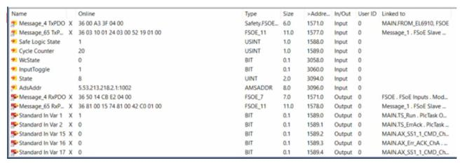
Here you can see that the connection between the EL6910 project and the Safe Motion project is working as configured.
