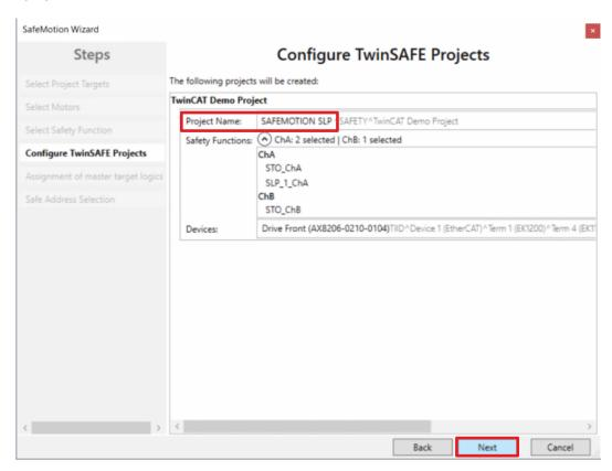
The "Configure TwinSAFE Projects" window opens. Here you have the option of renaming your Safe Motion project, which is generated for your Safe Motion component.
