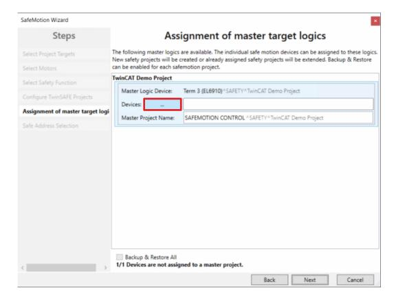
In the next window "Assignment of master target logics" the connection to the EL6910 project is closed, so that your Safe Motion component can communicate with the EL6910 project. The EL6910 project is automatically found and displayed.
