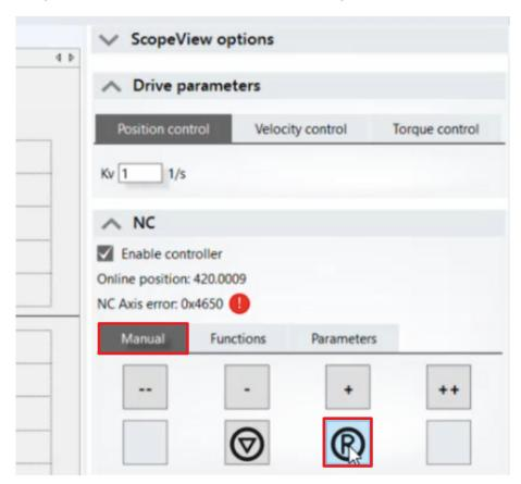
5. Click on the "R" symbol in the "Manual" tab to reset the error
