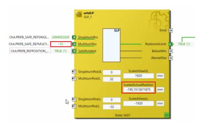
In the "ScaledActualPosition" field, you can see how the motor moves back and forth between -840 and 0 from a safety point of view.
