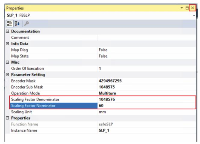
7. Enter the values from the Drive Manager for "Scale factor numerator" and "Scale factor denominator" in the corresponding lines
