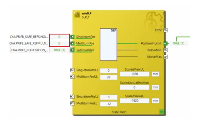
You will see that the current multiturn and singleturn position is set to 0 and the positions are therefore correctly configured.
