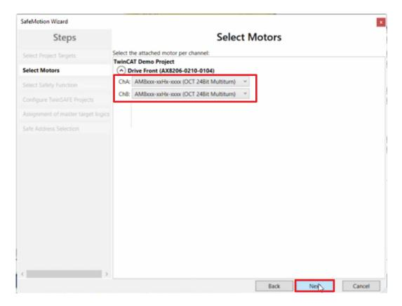
In the "Select Motors" window, configure the feedback for the individual axes.
