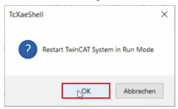
3. Confirm the "Restart TwinCAT System in Run Mode" window with "OK"
