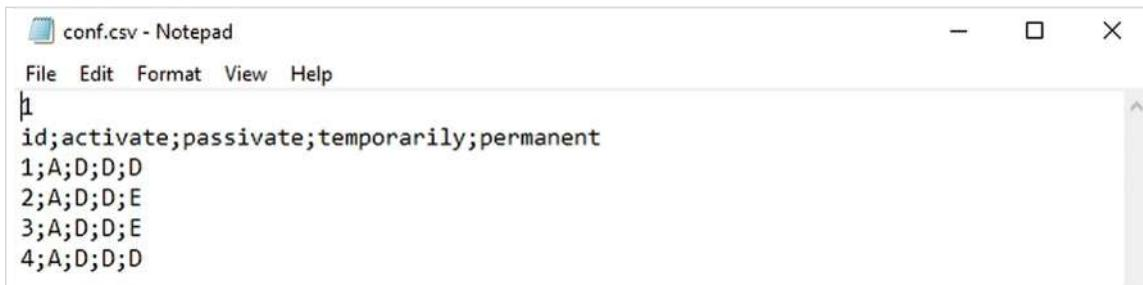
In the notepad, you can see the customizing settings for each of the 4 TwinSAFE groups. At the first group you can see for example at „A;D;D;D“, that the group is activated and no further settings for passivation or deactivation can be made.
