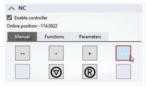
12. Click on the "++" symbol to move the motor manually into the plus range
