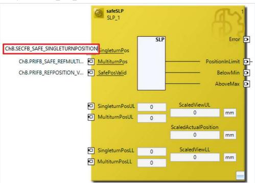
By default the first block processes the position of the Primary Feedback. Since the SLP functionality is to be implemented in the secondary feedback, adjust the function block as follows:
