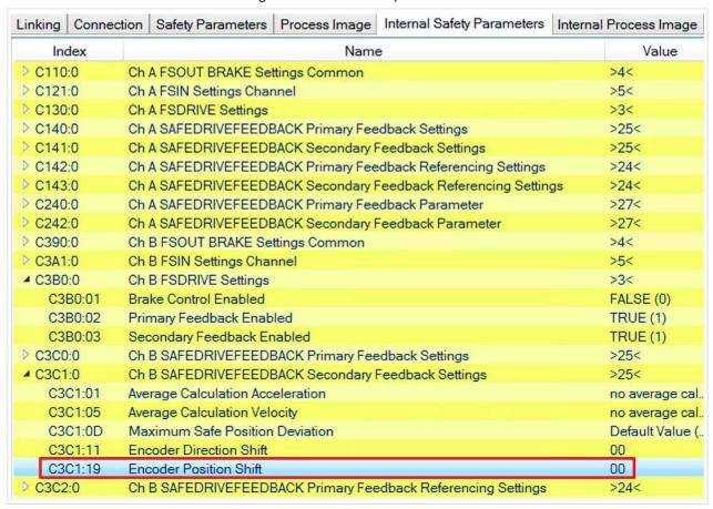
5. Double click on the parameter "C3C1:19 Encoder Position Shift"
