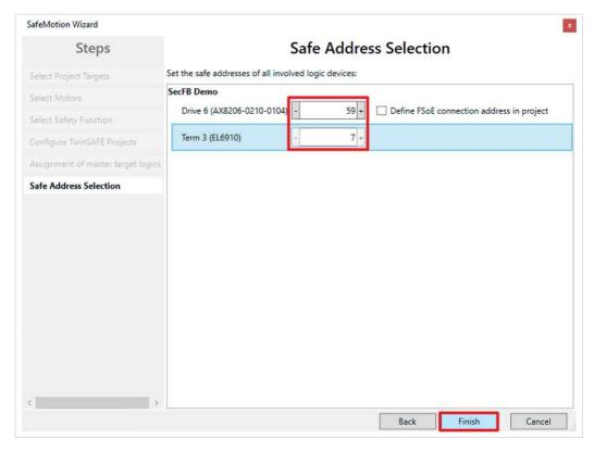
The "Safe Address Selection" window opens. Here the safe addresses are read out automatically. For virtual axes or axes that cannot be reached, you have the option of configuring the addresses yourself.
