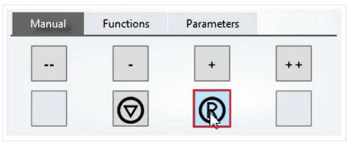
5. Click on the "R" symbol in the "Manual" tab to reset the error
