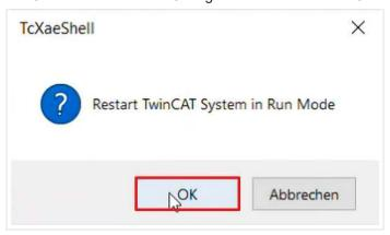
2. Confirm the "Restart TwinCAT System in Run Mode" window with "OK"
