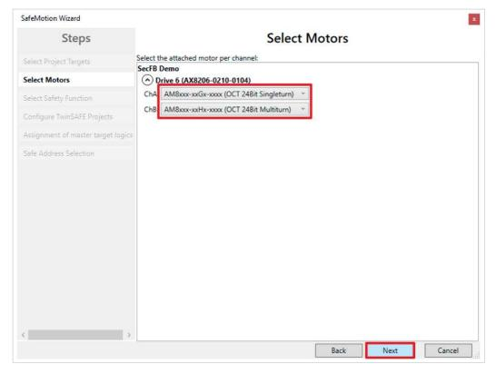
In the "Select Motors" window, you configure the feedback for the individual axes.
