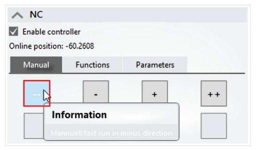
10. Click on the "—" symbol in the "Manual" tab to move the motor manually to the minus range
