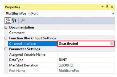
5. Select "Deactivated" in the drop-down menu of the channel interface to deactivate the input
