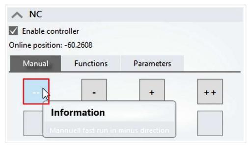
13. Click on the "—" symbol in the "Manual" tab to move the motor manually out of the permitted range
