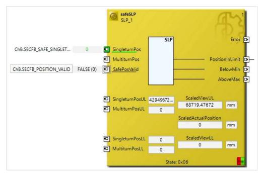
The signal for ChB.SECFB\_POSITION\_VALID is first displayed as FALSE, because more time is needed until the signal appears.
