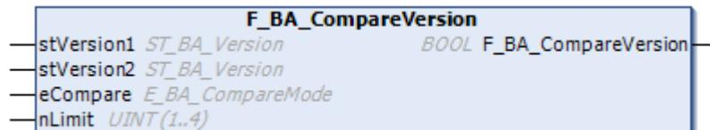
The function F\_BA\_CompareVersion of return type BOOL compares two version numbers *stVersion1* and *stVersion2*, each of type ST\_BA\_Version [► 78]. The input variable *nLimit* specifies how many digits are to be compared, starting with 1 = "Major". The enumeration *eCompare* specifies the comparison operation. The function return value changes to TRUE if the comparison is fulfilled.
