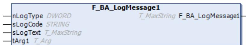
Internally the function FB\_BA\_LogMessage1 works with the function block FB\_FormatString.
