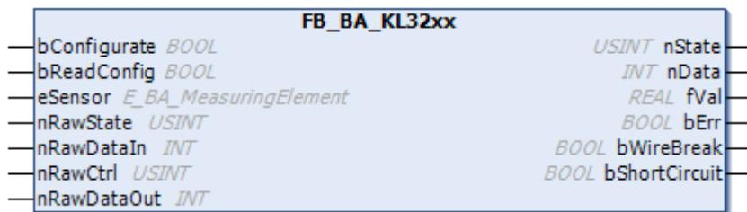
The function block FB\_BA\_KL32xx is for the configuration of Bus Terminals of the types KL3208\_0010, KL3201, KL3202 and KL3204.
