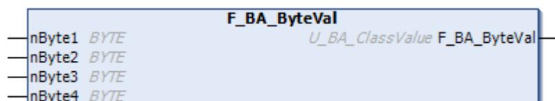
The return value of the F\_BA\_ByteVal function is created by the structure of type [U\\_BA\\_ClassValue \[► 80\]](#). The input values *nByte1*, *nByte2*, *nByte3* and *nByte4* are assigned in this structure on the respective values *nByteVal[1]*, *nByteVal[2]*, *nByteVal[3]* and *nByteVal[4]*. Due to the data type UNION, whose elements all start from the same memory address, all other values of this structure change as well.
