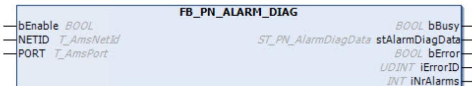
The function block FB\_PN\_ALARM\_DIAG can be used to read out diagnosis alarms. Each instance of this function block provides a PLC input ("PnIoBoxDiag"). This input must be linked to the "PnIoBoxDiag" input of the device to be evaluated. Once the diagnosis alarms/warnings have been successfully read, the alarm state of the device is reset. The function block must be called once for each PROFINET device. A run index (iNrAlarms) indicates how many diagnosis alarms have been read from the buffer.
