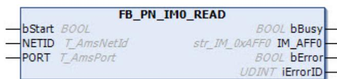
The PROFINET controller uses the function block FB\_PN\_Im0\_READ to read all I&M 0 ( Identification & Maintenance ) data from a device referenced via the input *Port*.
