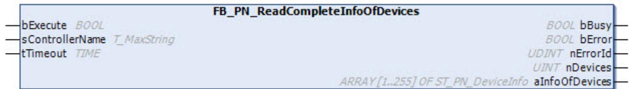
The function block FB\_PN\_ReadCompleteInfoOfDevices creates a list with the complete information of the configured devices (in TwinCAT). For PROFINET RT controllers such as TF6271 or CCAT M930 interface or EL6631 v11(v.024).
