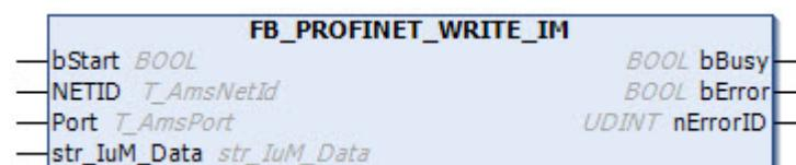
The function block FB\_PROFINET\_WRITE\_IM can be used to write the I&M (Identification & Maintenance) data of the respective PROFINET device.
