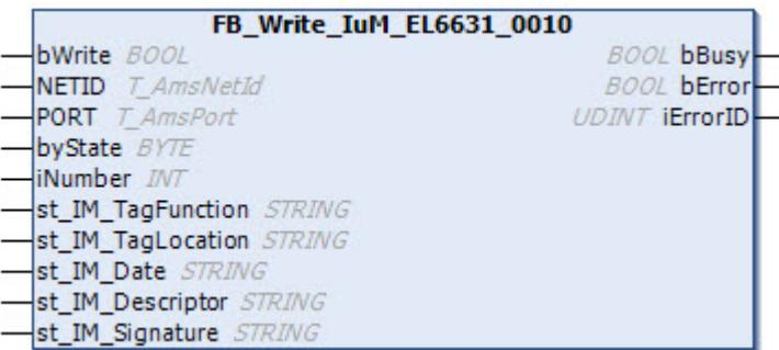
The function block FB\_Write\_IuM\_EL6631\_0010 writes I&M1, I&M2, I&M3 and I&M4 (Identification & Maintenance) data to the PROFINET device as a string via EtherCAT in accordance with the PROFINET specification.
