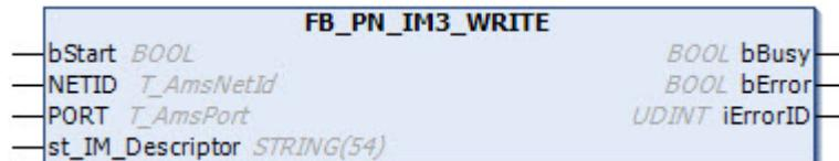
The PROFINET controller uses the function block FB\_PN\_IM3\_WRITE to write all I&M3 (Identification & Maintenance) data to a device referenced via the input *Port*.
