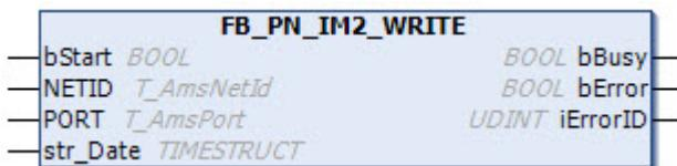
The PROFINET controller uses the function block FB\_PN\_IM2\_WRITE to write all I&M 2 (Identification & Maintenance) data to a device referenced via the input *Port*.
