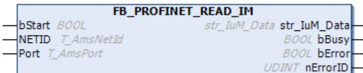
The function block FB\_PROFINET\_READ\_IM returns the I&M (Identification & Maintenance) data of the respective PROFINET device.
