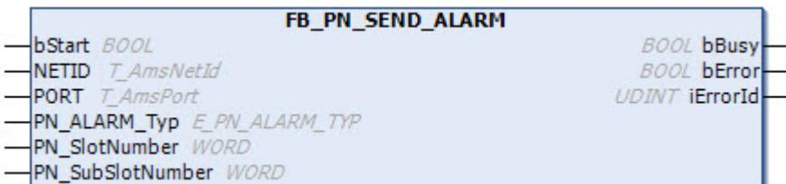
The function block FB\_PN\_SEND\_ALARM sends an alarm to the controller.
