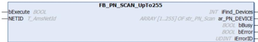
The FB\_PN\_SCAN\_UpTo255 function block scans the PROFINET network and returns the number of and a list with information on the PROFINET devices found.
