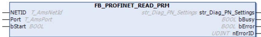
The function block FB\_PROFINET\_READ\_PRM scans the PROFINET network and returns the number and a list with information on the PROFINET devices found.
