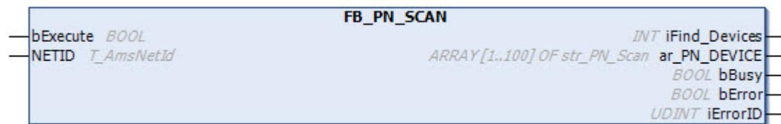
The function block FB\_PN\_SCAN scans the PROFINET network and returns the number and a list with information on the PROFINET devices found.
