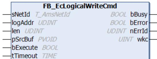
The master sends a logical EtherCAT write command (LWR) with the function block FB\_EcLogicalWriteCmd. In each slave, local address ranges (DPRAM) can be mapped to global logical address ranges. This command therefore addresses all EtherCAT slaves, which have mapping configured for the selected logical address range.
