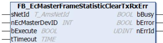
The function block `FB_EcMasterFrameStatisticClearTxRxErr` can be used to delete the error counters of the miniport driver of the network card.
