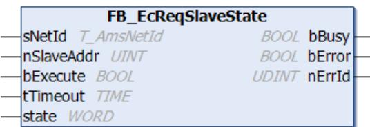
With this function block a slave can be set to a specified EtherCAT state. The requested EtherCAT state is transferred in the state variable. The function block becomes inactive as soon as it has sent the command to change state. Unlike the function block FB\_EcSetSlaveState it does not wait until the EtherCAT slave has attained the new state.
