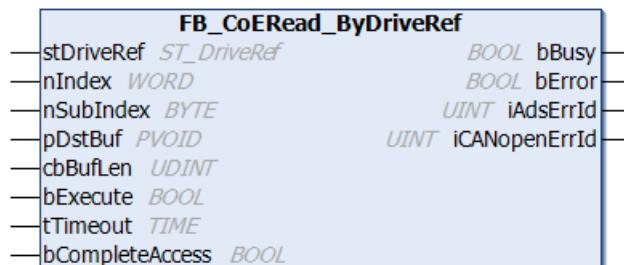
The function block `FB_CoERead_ByDriveRef` can be used to read drive parameters by means of the "CANopen over EtherCAT (CoE)" protocol. This requires the slave to have a mailbox and to support the "CANopen over EtherCAT" (CoE) protocol. The `nSubIndex` and `nIndex` parameters allow the object that is to be read to be selected. Via `bCompleteAccess := TRUE` the parameter can be read with subelements.
