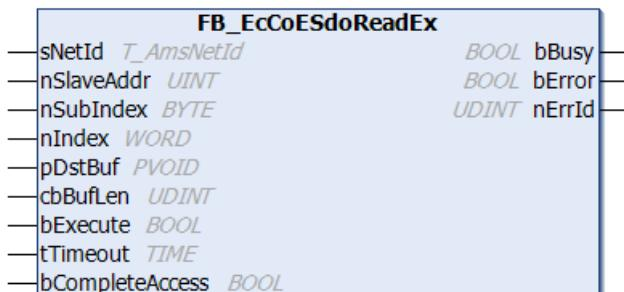
The **FB\_EcCoESdoReadEx** function block allows data to be read from an object dictionary of an EtherCAT slave through an SDO (Service Data Object) access. This requires the slave to have a mailbox and to support the “CANopen over EtherCAT” (CoE) protocol. The nSubIndex and nIndex parameters allow the object that is to be read to be selected. The parameter with subelements can be read via bCompleteAccess := TRUE.
