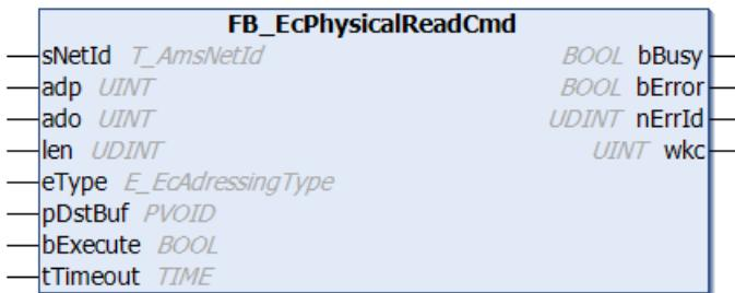
The function block `FB_EcPhysicalReadCmd` can be used to send an EtherCAT read command (FPRD, APRD, BRD) to a particular EtherCAT slave or to all EtherCAT slaves. This command can be used by the PLC to read a register or the DPRAM of the EtherCAT slave controller.
