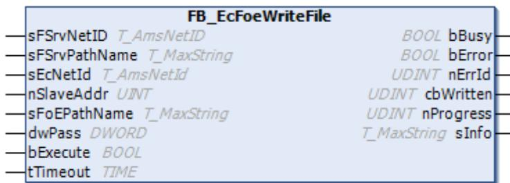
The function block FB\_EcFoeWriteFile can be used to write files from a local data carrier to an EtherCAT device via the "File access over EtherCAT" mailbox protocol.
