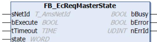
With this function block the EtherCAT state of a master device can be requested and set. The requested EtherCAT state is transferred in the state variable. The function block becomes inactive as soon as it has requested the EtherCAT state. Unlike the function block FB\_EcSetMasterState it does not wait until the new state is set.
