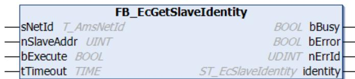
The function block **FB\_EcGetSlaveIdentity** can be used to read the CANopen identity of an individual EtherCAT slave device. If the call is successful, the output variable **identity**, whose type is **ST\_EcSlaveIdentity**, contains the requested identity information.
