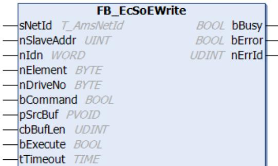
The function block **FB\_EcSoeWrite** can be used to write drive parameters by means of the “Servo drive profile over EtherCAT (SoE)” protocol. To this end the slave must have a mailbox and support the SoE protocol. The drive parameter to be written is specified with the parameters nIdn (identification number), nElement and nDriveNo.
