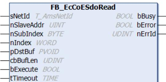
The **FB\_EcCoeSdoRead** function block allows data to be read from an object dictionary of an EtherCAT slave through an SDO (Service Data Object) access. This requires the slave to have a mailbox and to support the “CANopen over EtherCAT” (CoE) protocol. The nSubIndex and nIndex parameters allow the object that is to be read to be selected. The function block [FB\\_EcCoeSdoReadEx \[▶ 50\]](#) must be used for access to the complete parameter, including subelements.
