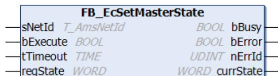
With this function block the EtherCAT state of a master device can be requested and set. The requested EtherCAT state is transferred with the **reqState** variable. The function block requests the EtherCAT state and, unlike the function block **FB\_EcReqMasterState**, remains active until the new state is set or the maximum time **tTimeout** is exceeded. The current state is output in the **currState** variable.
