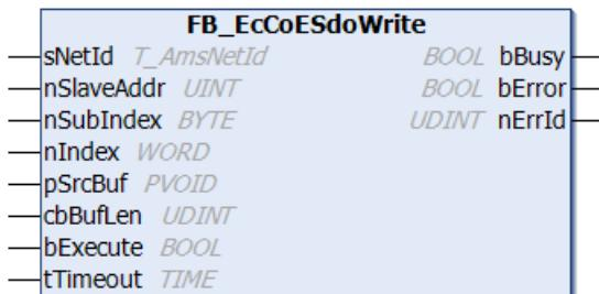
The **FB\_EcCoeSdoWrite** function block permits an object from the object directory of an EtherCAT slave to be written by means of an SDO download. This requires the slave to have a mailbox and to support the "CANopen over EtherCAT" (CoE) protocol. The nSubIndex and nIndex parameters allow the object that is to be written to be selected. The function block **FB\_EcCoeSdoWriteEx** [▶ 53] must be used for access to the complete parameter, including subelements.
