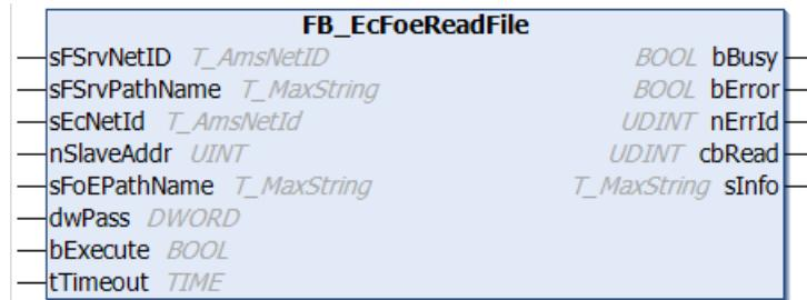
The FB\_EcFoeReadFile function block can be used to download files from an EtherCAT device to the local data carrier via the "File access over EtherCAT" mailbox protocol.
