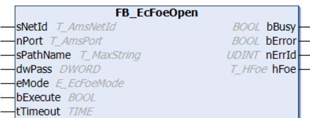
This function block is used to open the communication port for the “File access over EtherCAT” mailbox protocol.
