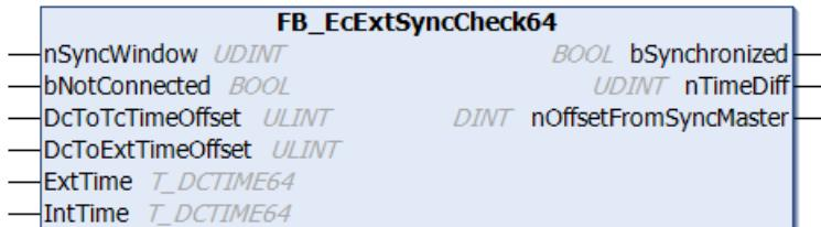
The function block **FB\_EcExtSyncCheck64** checks whether the internal and external clocks are synchronous. See function block **FB\_EcExtSyncCalcTimeDiff64** [▶ 96].
