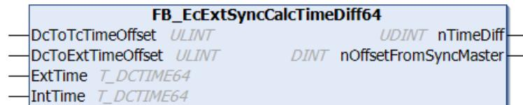
The function block `FB_EcExtSyncCalcTimeDiff64` calculates the difference between external and internal time, taking into account the time offsets.
