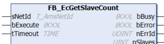
The function block `FB_EcGetSlaveCount` can be used to determine the number of slaves that are connected to the master.
