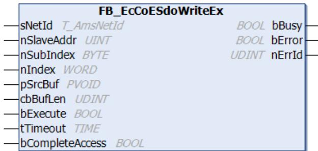
The FB\_EcCoeSdoWriteEx function block permits an object from the object directory of an EtherCAT slave to be written by means of an SDO download. This requires the slave to have a mailbox and to support the "CANopen over EtherCAT" (CoE) protocol. The nSubIndex and nIndex parameters allow the object that is to be written to be selected. Via bCompleteAccess := TRUE the parameter can be written with sub-elements.
