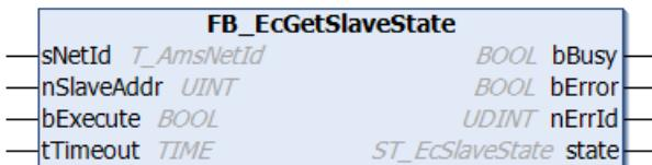
The function block **FB\_EcGetSlaveState** allows the EtherCAT status and the Link status of an individual EtherCAT slave to be read. If the call is successful, the output variable **state**, whose type is **ST\_EcSlaveState**, contains the requested status information.
