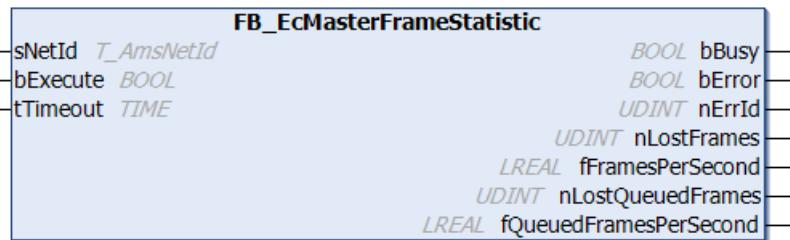
The function block `FB_EcMasterFrameStatistic` can be used to read the frame statistics of the EtherCAT master. A distinction is made between cyclic and acyclic (queued) frames. Acyclic frames are used for the initialization or for parameter access to EtherCAT slaves. Frames are regarded as lost if they fail to return to the master or are invalid.
