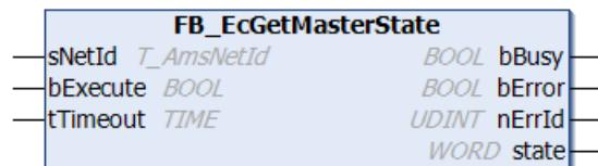
The function block **FB\_EcGetMasterState** can be used to read the EtherCAT state of the master. If the call is successful, the **State** output variable of type WORD contains the requested status information.
