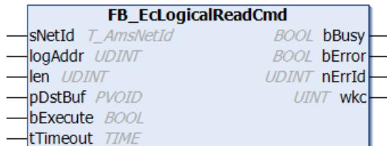
The master sends a logical EtherCAT read command (LRD) with the function block **FB\_EcLogicalReadCmd**. In each slave, local address ranges (DPRAM) can be mapped to global logical address ranges. This command therefore addresses all EtherCAT slaves, which have mapping configured for the selected logical address range.
