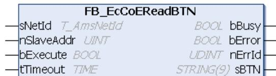
The function block FB\_EcCoeReadBTN can be used to read the BTN from the object directory of an EtherCAT slave via SDO (Service Data Object) access. For this the slave must have a mailbox and support the "CANopen over EtherCAT (CoE)" protocol and the object directory must contain an object 0xF083 with the BTN.
