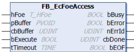
This function block writes or reads data via the communication port of the “File access over EtherCAT” mailbox protocol.
