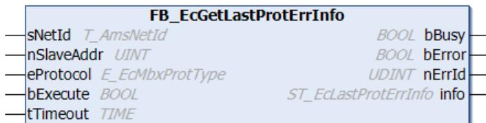
The function block **FB\_EcGetLastProtErrInfo** can be used to read additional error information relating to the most recent mailbox protocol error. An error-free mailbox command resets the last error every time.
