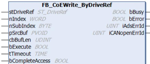
The function block **FB\_CoEWrite\_ByDriveRef** can be used to write drive parameters based on the "CANopen over EtherCAT (CoE)" protocol. This requires the slave to have a mailbox and to support the "CANopen over EtherCAT" (CoE) protocol. The nIndex and nSubIndex parameters allow the object that is to be written to be selected. Via bCompleteAccess := TRUE the parameter can be written with sub-elements.
