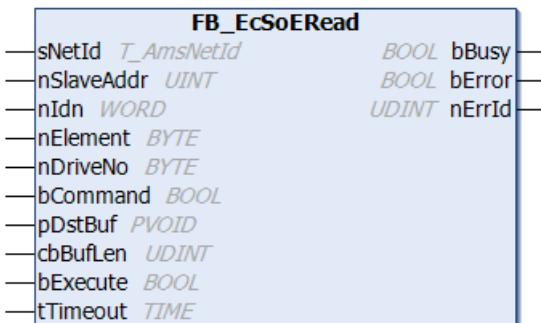
The function block **FB\_EcSoeRead** can be used to read drive parameters by means of the “Servo drive profile over EtherCAT (SoE)” protocol. To this end the slave must have a mailbox and support the SoE protocol. The drive parameter to be read is specified with the parameters nIdn (identification number), nElement and nDriveNo.
