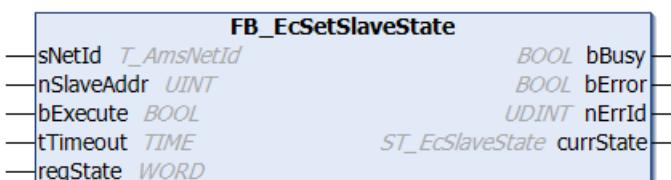
With this function block a slave can be set to a specified EtherCAT state. The requested EtherCAT state is transferred with the reqState variable. The function block sends the command to change state and, unlike the function block FB\_EcRegSlaveState, remains active until the EtherCAT slave has attained the new state or the maximum time tTimeout is exceeded. The current state is output in the currState variable.
