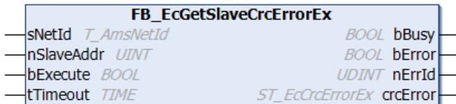
The function block `FB_EcGetSlaveCrcErrorEx` allows the CRC error counters of the individual ports (A, D, B and C) of a slave to be read. If the call is successful, the output variable `crcError`, whose type is `ST_EcCrcErrorEx`, contains the requested CRC error counter.
