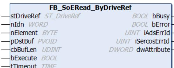
The FB\_SoeRead\_ByRef function block can be used to read drive parameters by means of the “Servo drive profile over EtherCAT (SoE)” protocol. To this end the slave must have a mailbox and support the SoE protocol. The drive parameter to be read is specified with the parameters nIdn (identification number), nElement and stDriveRef.
