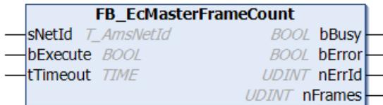
The function block `FB_EcMasterFrameCount` can be used to determine the number of EtherCAT frames configured in the master.
