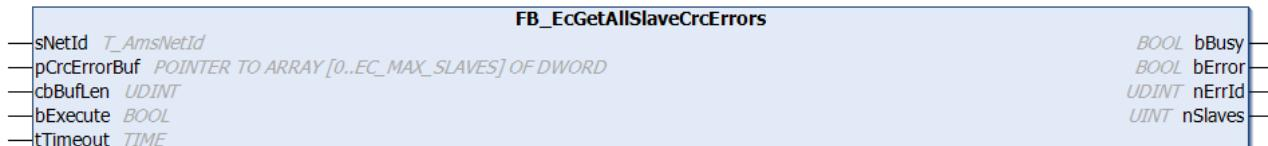
The **FB\_EcGetAllSlaveCrcErrors** function block allows the CRC error counters of all the slaves connected to the master to be read. The CRC errors at the individual ports of a slave are added.
