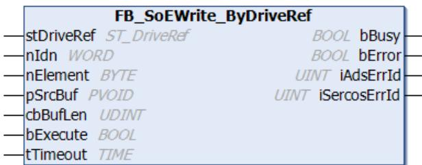
The function block `FB_SoEWrite_ByRef` can be used to write drive parameters by means of the “Servo drive profile over EtherCAT (SoE)” protocol. To this end the slave must have a mailbox and support the SoE protocol. The drive parameter to be written is specified with the parameters `nIdn` (identification number), `nElement` and `stDriveRef`.
