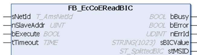
The function block FB\_EcCoeReadBIC can be used to read the BIC from the object directory of an EtherCAT slave via SDO (Service Data Object) access. For this the slave must have a mailbox and support the "CANopen over EtherCAT (CoE)" protocol and the object directory must contain an object 0x10E2:01 with the BIC.
