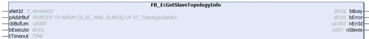
The function block **FB\_EcGetSlaveTopologyInfo** can be used to determine topology information.
