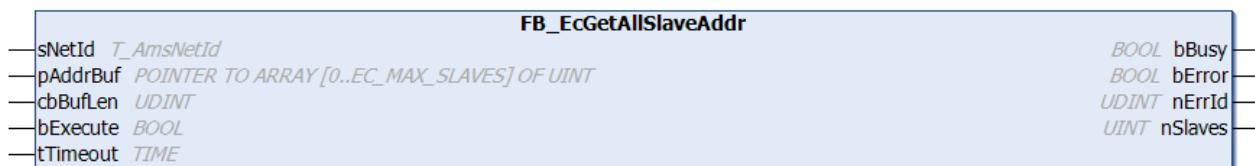
The **FB\_EcGetAllSlaveAddr** function block allows the addresses of all the slaves connected to the master to be read. When the call is successful, the buffer passed in the parameter **pAddrBuf** contains the addresses of all the slaves as an array of **UINTs**.
