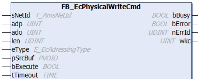
The function block **FB\_EcPhysicalWriteCmd** can be used to send an EtherCAT write command (FPWR, APWR, BWR) to a particular EtherCAT slave or to all EtherCAT slaves. This command can be used by the PLC to write to a register or the DPRAM of the EtherCAT slave controller.
