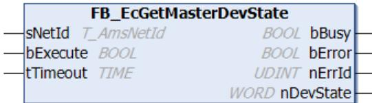
The function block **FB\_EcGetMasterDevState** can be used to read the current state of the EtherCAT master.
