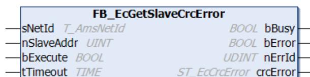
The function block `FB_EcGetSlaveCrcError` allows the CRC error counters of the individual ports (A, B and C) of a slave to be read. If the call is successful, the output variable `crcError`, whose type is `ST_EcCrcError`, contains the requested CRC error counter.
