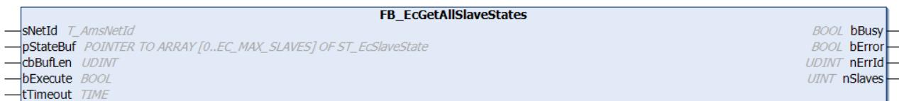
The **FB\_EcGetAllSlaveStates** function block allows the EtherCAT status and the Link status of all the slaves connected to the master to be read. When the call is successful, the buffer passed in the parameter **pStateBuf** contains the requested status information as an array of **ST\_EcSlaveState**.
