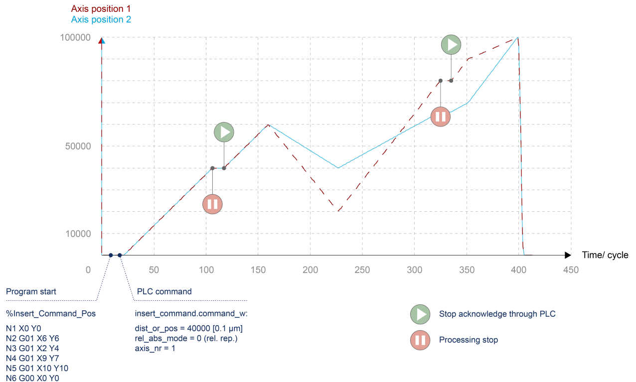
Fig. 4: STOP mark command at standstill with axis position reached multiple times
