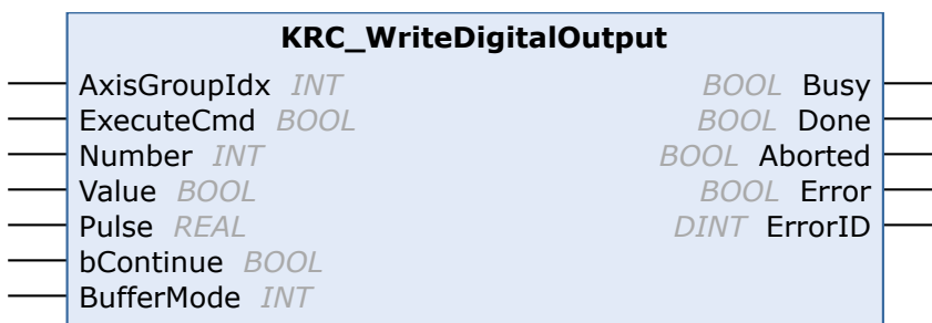
Fig. 86: Function block KRC_WriteDigitalOutput
