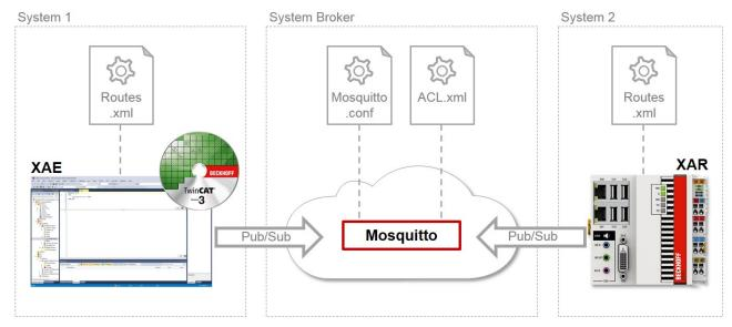
The configuration files listed in the illustration must be created and adapted accordingly in order to use ADS-over-MQTT. Two examples are presented below.
