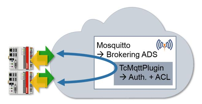
The plugin is supplied with the TwinCAT installation and is located in the folder *C:* \TwinCAT\AdsApi\TcMqttPlugin or C:\TwinCAT\AdsApi\x64\TcMqttPlugin if a 64-bit Mosquitto Broker is used. The plugin is integrated in the Mosquitto configuration as follows:
