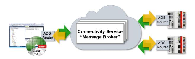
This document provides an overview of the usage possibilities as well as a technical description of how a "virtual ADS network" can be configured over an MQTT message broker.
