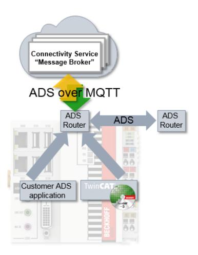
The ADS applications use ADS routes to identify the communication partner. This ADS route is independent of the transport channel and is described in the TwinCAT router.
