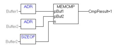
In this example, 4 bytes of data in *Buffer2* are compared with those in *Buffer1*. The first differing byte is larger in *Buffer1* than it is in *Buffer2*.
