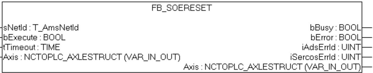
The functionblock FB\_SoEReset can be used to execute a drive reset (S-0-0099). Drives with more than on channel may require a reset on all channels. The timeout time must be 10s, because the reset can take up to 10s.
