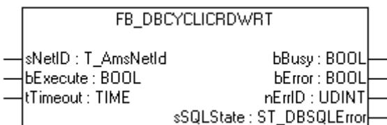
The FB\_DBCyclicRdWrt function block can be used to start or stop the cyclic logging \ writing of variables.
