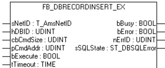
The FB\_DBRecordInsert\_EX function block allows individual data records to be written into a database. The length of the SQL - command could be till 10000 symbols. For using this function block you have to declare the database, you want to write to, in the XML - configuration file.
