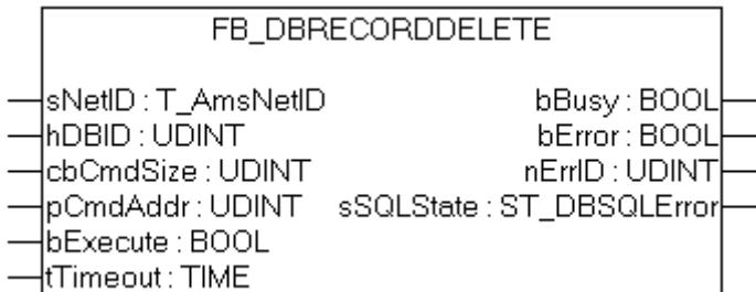
The FB\_DBRecordDelete function block allows to delete data records out of a database. The length of the SQL - command could be till 10000 symbols. For using this function block you have to declare the database, you want to delete from, in the XML - configuration file.
