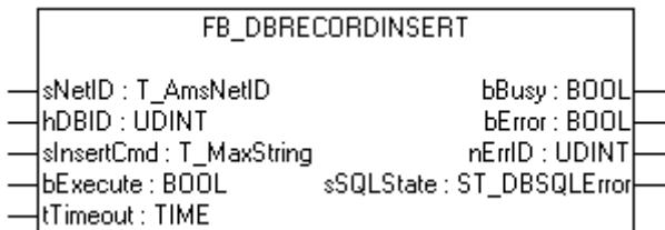
The FB\_DBRecordInsert function block allows individual data records to be written into a database. For using this function block, you have to declare the database, you want to write to, in the XML - configuration file.
