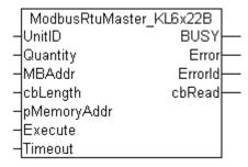
The function block *ModbusRtuMaster\_KL6x22B* implements a Modbus master that communicates via a serial Bus Terminal KL6021 or KL6041. The block is not called in its basic form, but individual actions of that block are used within a PLC program. Each Modbus function is implemented as an action.
