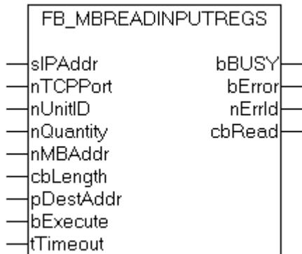
This function is used for reading 1 to 128 input registers (16 bit). Endian
