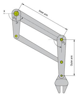
The 2-D-kinematics type 3 is built up as shown in the schema above.
