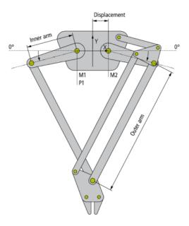
The 2-D-kinematics type 1 is built up as shown in the schema above.
