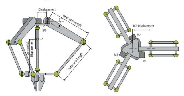
The delta kinematics type 1 is built up as shown in the schema above. The kinematic transformation expects ball joints (or elements with the same behavior) in the connection of the arms and to the lower plate.
