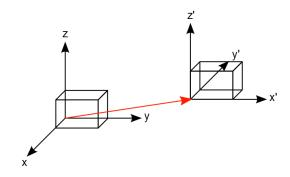
The static transformation supports a translation and rotation. By using this transformation, it is possible to define a User Coordinate System (UCS). This module takes care of the transformation from UCS to the Machine Coordinate System (MCS).
