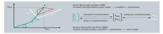
All ACS and MCS axes that are used in a kinematic transformation channel must be created in the System Manager. So for example a Delta-Robot will have 3 ACS axes (M1...M3) and 3 MCS axes (X, Y, Z).
