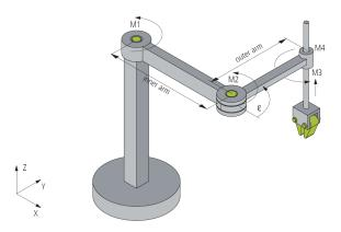
The SCARA (Selective Compliance Assembly Robot Arm) kinematics is built up as shown in the schema above.
